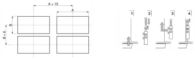
To assemble several instruments side-by-side, make sure axle bases are correct, as shown in the drawing. Dimensions A and B can be read in the overall dimensions indicated in the manual.
