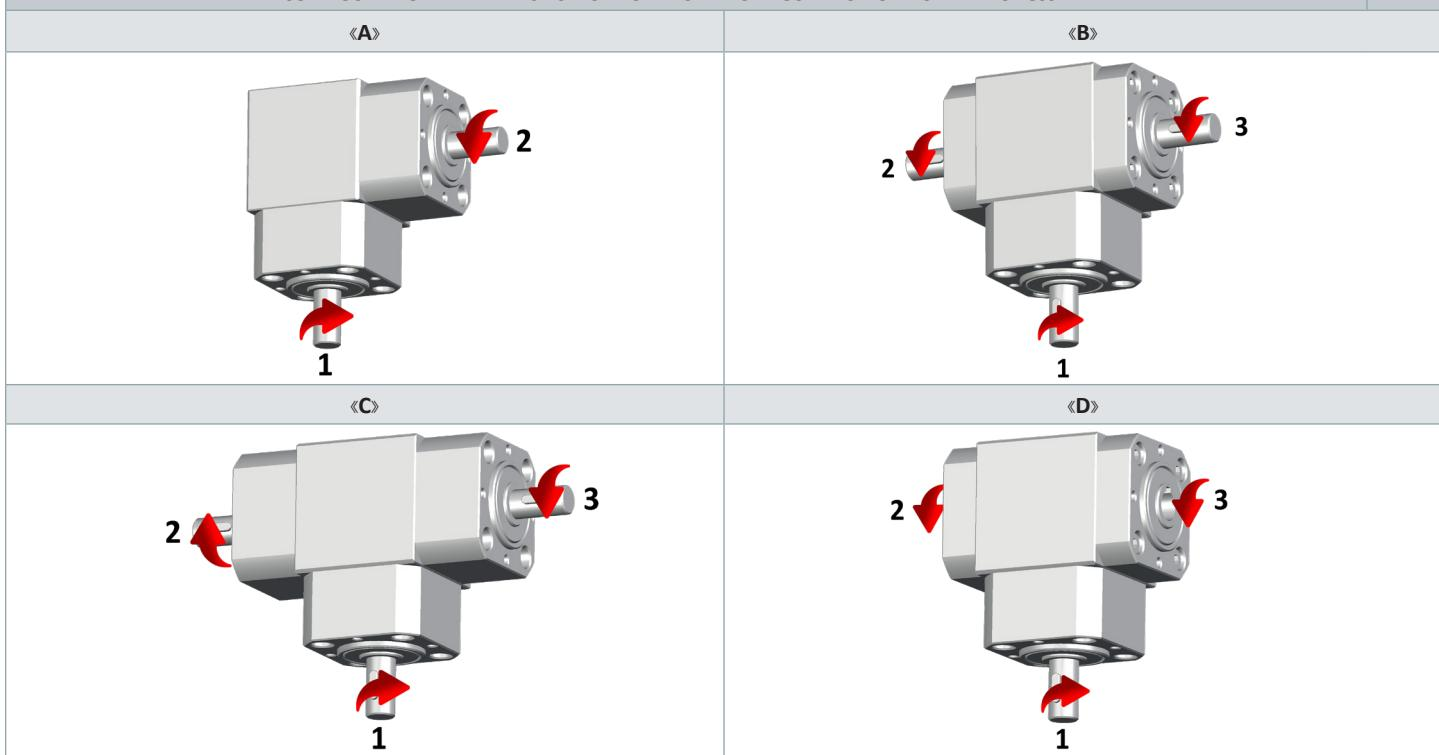
The direction of rotation depends from the configuration and from the positioning; see "Versions with dimension drawings" (Tab. 9).
