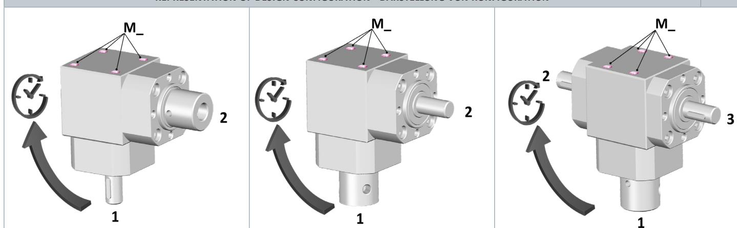
The desing configuration is determined by the shaft **1** always shown on the opposite side of the fixing bores **M\_**, the others shaft are defined following the clockwise direction (see "Part nr. configuration").
