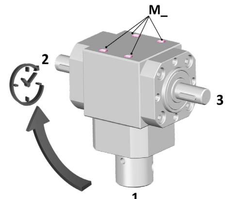
The design configuration is determined by the shaft <1> always shown on the opposite side of the fixing bores **M-**, the other shafts are defined following the clockwise direction (see "Part nr. configuration").
